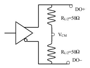
Figure 19. DC Output Reference System Load
