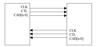
Figure 1. HyperTransport<sup>TM</sup> I/O Link
