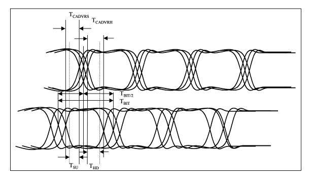
Figure 35. Reconciling Link Transfer Timing
