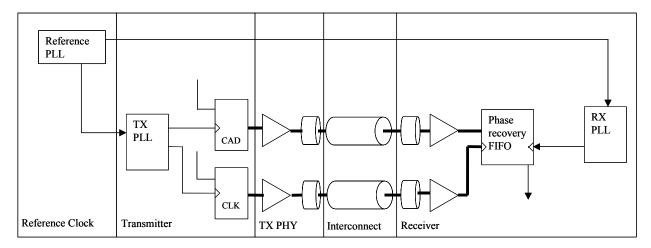
Figure 36. Representative Transmitter and Receiver
