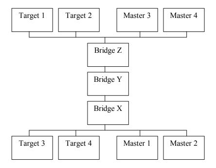
Figure 14. Example PCI System
