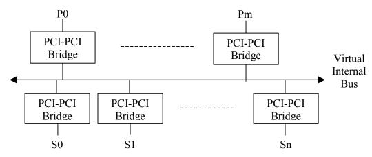
Figure 17. Logical Model of a Switch
