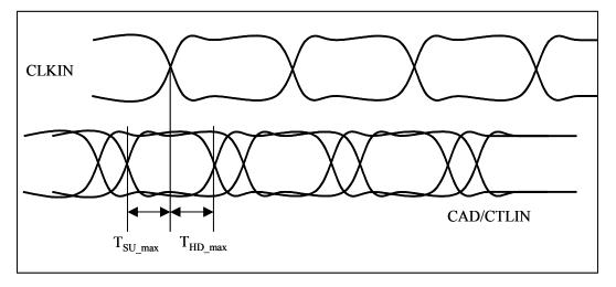
Figure 33.  $T_{SU}$  and  $T_{HD}$
